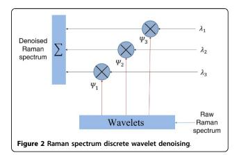
(c) wavelet transformation, widely used in the field of signal processing [24,25]. However, for Raman spectrum with complicated background noise, these methods might not work well, possibly requiring certain user interference or taking a long time. In this study we have developed an automatic piecewise fitting method for Raman baseline correction.
