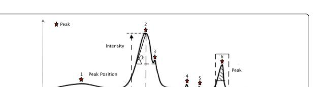
Figure 3 Principles for Raman spectrum discretization. Stars represent peaks, and dashed boxes represent windows.
