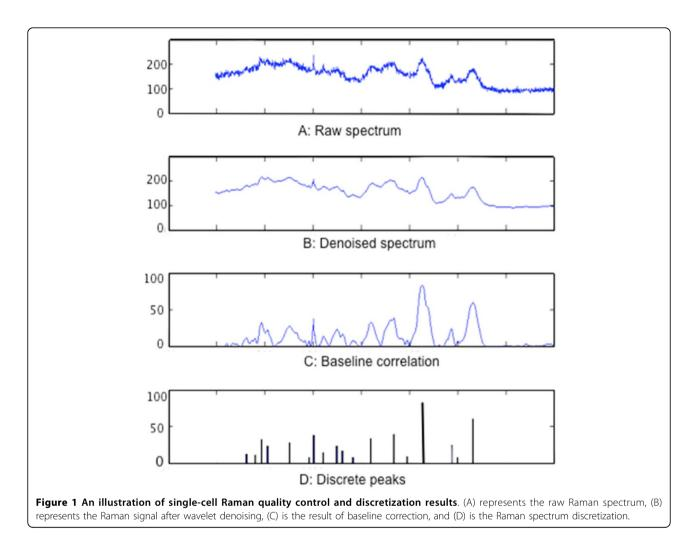
discrete wavelet transform for noise reduction in this study (Figure 2). As shown in Figure 1(B), the denoised Raman signal by discrete wavelet transform is smoother and still retains most significant features of Raman signals.
